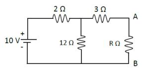
3. Determine the mesh currents for the circuit shown below.
