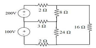
4. Use nodal analysis to find the node voltages for the below circuit.
